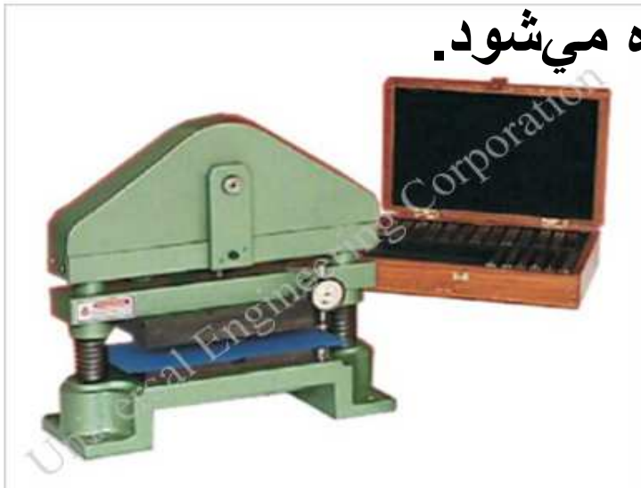
Carton board creaser is used to test the crease ability of carton board
